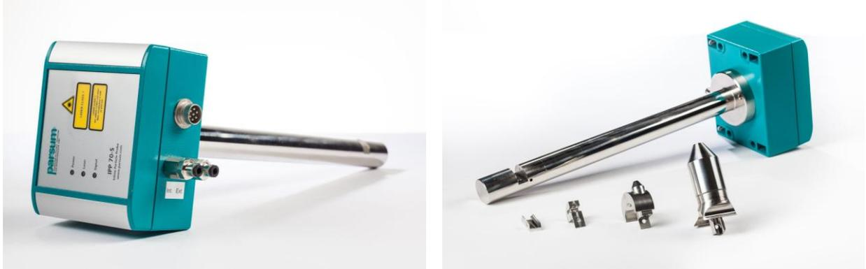
The IPP 70-S is used to monitor the target fraction downstream of the classifying screen and is situated directly behind the classifier at the outlet. The ATEX-certified IPP 70-Se has been installed directly in the process chamber for in-process checks and tracks the course of the process by constantly measuring the particle-size distribution.
