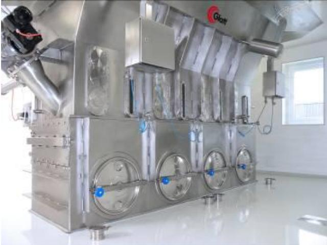
The process chamber of the GFG 250 is approximately 3.5 m long, 0.8 m wide and 0.7 m high. The hold-up is between 200 and 700 kg, depending on the product and method.
