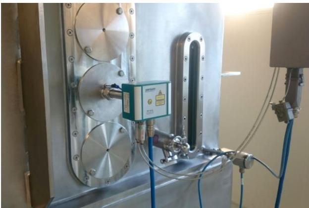
IPC is very happy with the use of the Parsum probes: “The continuous checking and monitoring of particle size during the process allows us to adjust the process parameters according to the desired target specification so as to achieve an optimal result,” says Demian. “By monitoring the target fraction, we can detect deviations from the desired result early and react quickly to protect the process.”
