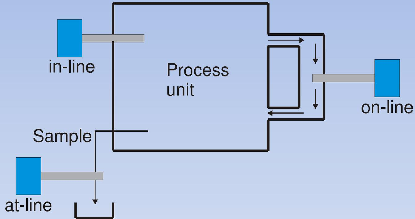
**Focus: Examples of in-line particle sizing**
