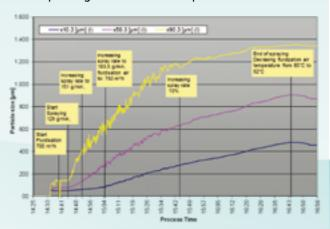
**Continuous agglomeration** – Measurement after a rotary valve in the continuous agglomeration of detergent. Inline particle measurement shortens the start-up phase and helps the operator keep the process stable.
