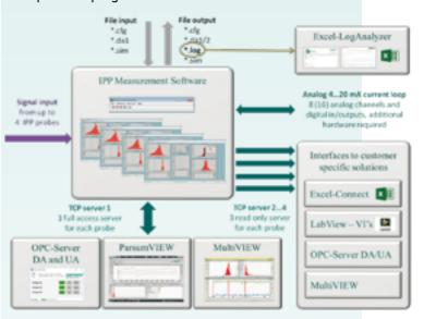
IPP - This is the measurement program proper that is the core of the software. It is designed to control the measurement and to provide a clear presentation of the results.
