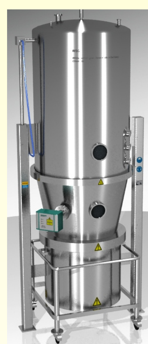
In-line measurement with probe IPP 70 for batch fluidized bed granulation
